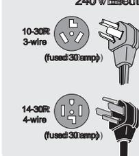
UL-approved electrical cord must be installed on electrical dryers (as not provided with unit except those manufactured outside in Canada).
